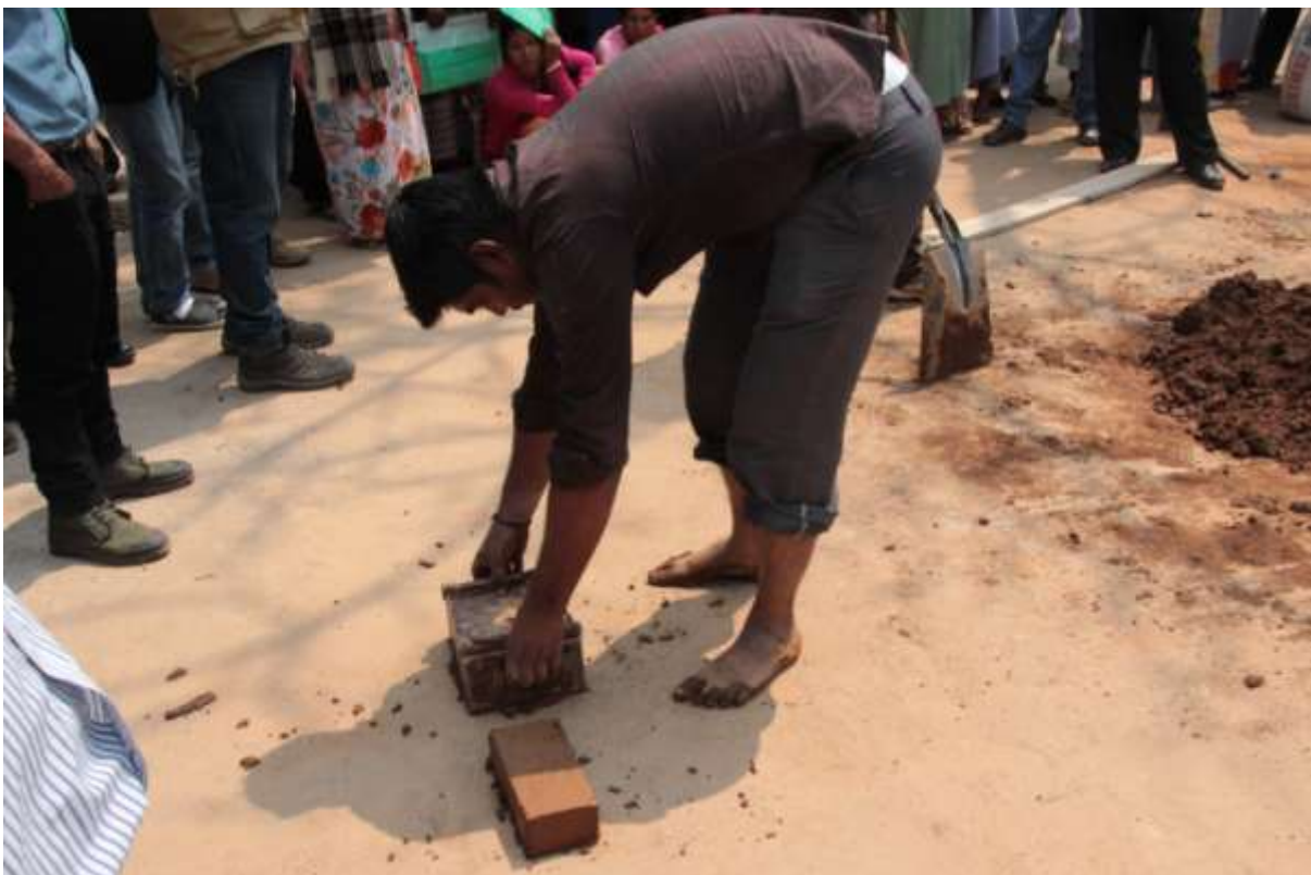
Picture 11 The block is then emitted from the mould by overturning it on a flat surface. This is then left for one day, before it is lifted and stacked for curing.
