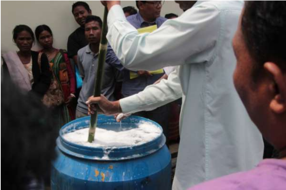
Picture 18 A session on the preparation of the Borax chemical solution used for the treatment of the bamboos.
