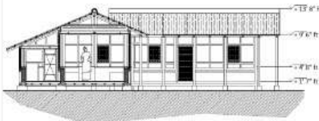
Drawing 2: Section through the House and extension
