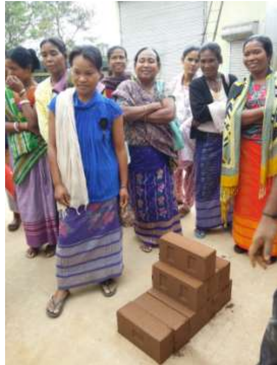
Picture 13 Compressed Earth Stabilised Blocks made from the Mardhini press
